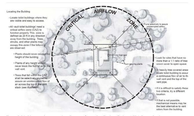
Figure 3.94 Diagram demonstrating distances for vault toilet installation. USDA Forest Service, Technology and Development Program. SST Installation Guide. 0323–1303. May 2003.
