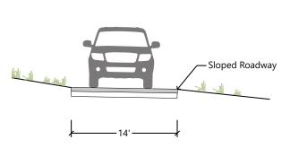
Figure 3.36 Secondary roads should be paved and designed to drain away from campsites.
