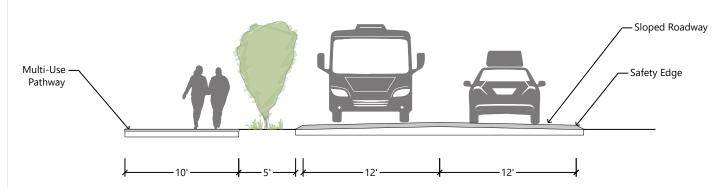
Figure 3.35 Section of vehicular road with cars, pedestrians, and buffer.
