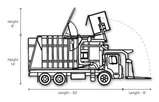
Figure 3.34 When using dumpsters, consider the overall size and operational height of collection vehicles.
