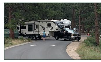
Figure 3.37 Two images show a truck with a fifth-wheel trailer cutting over a radius that's too small in order to back into a campsite. In this case, a gravel buffer was added to extend the road width without additional asphalt. This assists the driver by providing a widened radius section and protects plant resources on the edge of the road.
