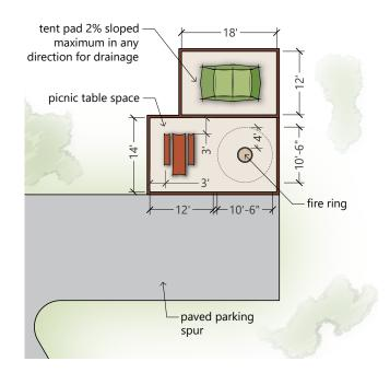
Figure 3.58 12' x 18' Campsite with tent pad, picnic table, fire ring, and paved parking spur.
