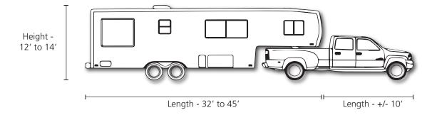
Figure 3.33 Consider total height and length of tow vehicle in addition to trailer.
