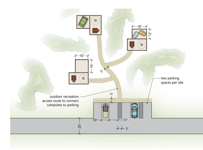
Figure 3.66 Accessible walk-in campsite with parking stalls, walkways to three campsites, and a comfort station.
