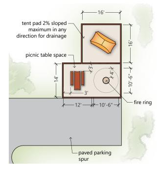
Figure 3.57 16' x 16' Campsite with tent pad, picnic table, fire ring, and paved parking spur.
