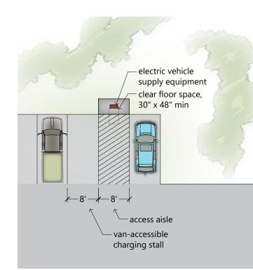
Figure 3.130 Plan view of a van-accessible charging stall.
