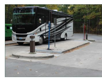
Figure 3.125 Sleeping Bear Dunes National Lakeshore, Michigan, Platte River. Campground dump station includes an accessible RV parking lane with island access aisle to approach station components.
