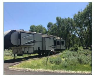
Figure 3.62 Numerous camper slide outs add room to the interior of the camper but require additional space on the exterior.
