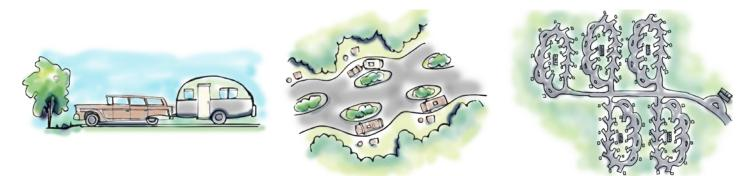
Figure 1.5 1950s. Mission 66 (1956) ushered in new campground design. This included large, multi-loop road campgrounds; large parking spurs or pull-through turnouts for parking; large campsites; mass-produced picnic tables; and fire grates/grills at each campsite. Group amenities were also provided.
