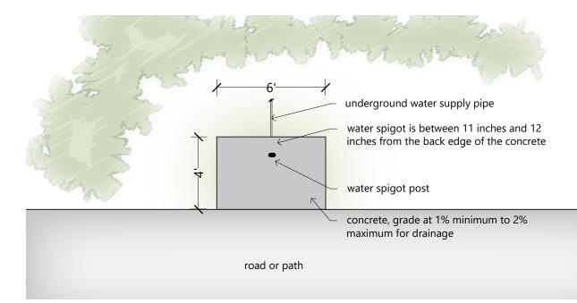
Figure 3.82 Accessible water spigot in plan view.
