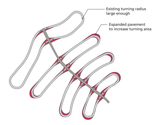
Figure 3.38 Existing one-way loops shown in gray. Expanded pavement shown in red provides additional area to accommodate larger turning radius. Additional area can be expanded on the outside or inside of a curve. An engineer will determine what is most feasible.
