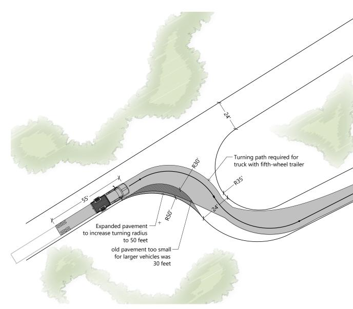
Figure 3.32 Larger radii are needed to accommodate larger vehicles. In situations where the roadway is narrow, the curves will need to be widened or hardened with gravel to allow vehicles to make safe turning movements.
