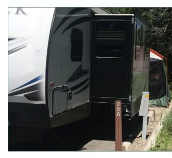
Figure 3.99 Many camper slide outs are located on the same side as the utility hookups. For this reason, additional protection is needed to prevent a camper for inadvertently damaging utilities.
