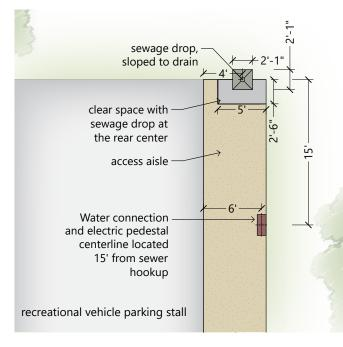
Figure 3.86 Accessible approach to sewer hookup.
