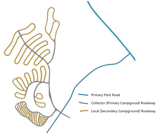
Figure 3.31 The hierarchical road system aids in wayfinding for visitors. Roads designed for campground areas must provide adequate dimensions for the largest vehicle allowed and/or expected to use the campground or specific location within the campground. However, the general desire in most NPS campgrounds will be to design campground roads in a manner that requires a slower speed with less formal shoulder areas than may be found on the main park road.
