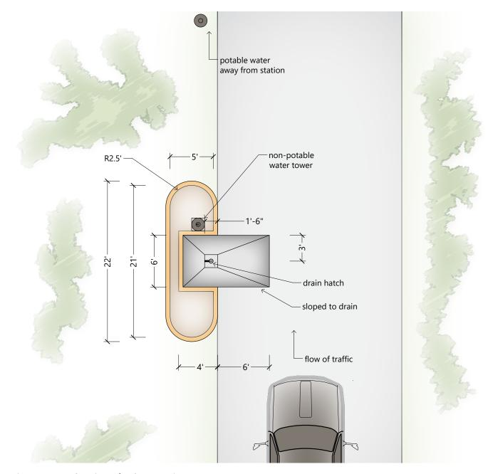
Figure 3.126 Plan view of a dump station.
